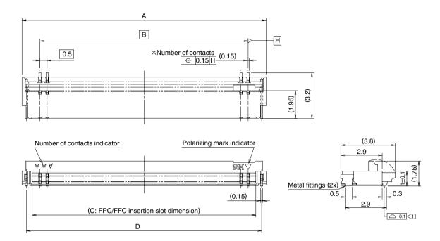
Note  $\boxed{1}$ : The coplanarity of each terminal lead is within 0.1.
