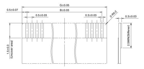
\*Polyimide and thermally hardening adhesive is recommended as the materials for the stiffener. Note: When using the FPC/FFC in FH34S or FH19SC connectors, the exposed area inserted in either connector is 2.5mm  $\pm$  0.3mm and the stiffener is 3.5mm min.
